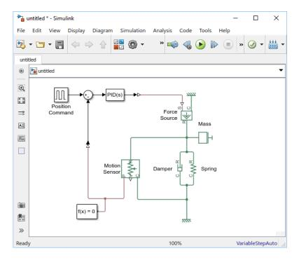
The control Simulink signal goes to the input port of the Simulink-PS Converter block, where it is converted into a physical signal driving the force profile of the Ideal Force Source block.
