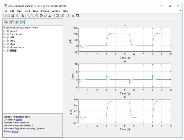
Expand the Spring node and select node x. The right pane displays the spring deformation data plotted over time.
