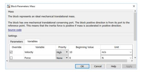
Note that the **Override** check box next to the **Velocity** variable is now selected, which means that you have overridden the default variable initialization value. This variable has high priority, therefore, the solver will try to exactly satisfy this beginning value when it computes the initial conditions to determine the simulation starting point.
